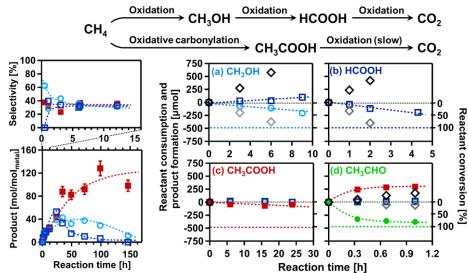
Reaction mechanism investigation of CO-assisted methane partial oxidation over Rh-ZSM-5 catalyst
