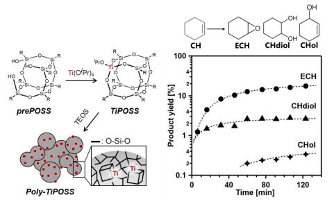
Nanoporous titanosilicate catalyst synthesized from siloxane precursor molecule possessing 4-coordinated Ti species *Nanoscale*, 15, 9792 (2023)
